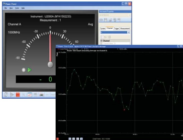
Figure 4 Strip chart continuous analog monitor of a power channel.
