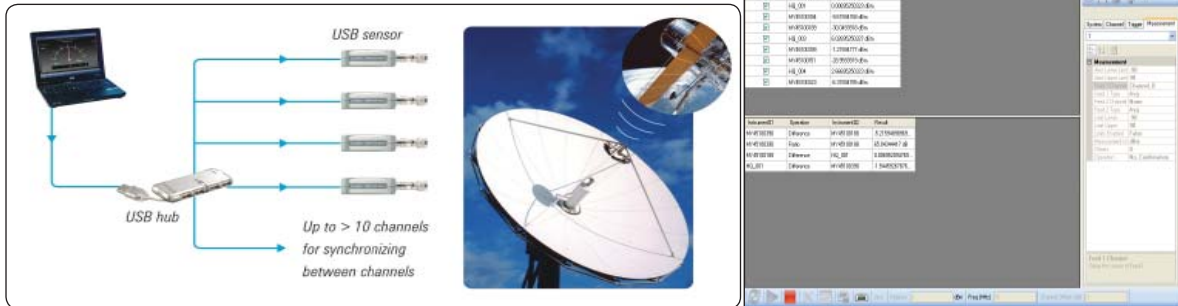
Figure 14 By multiplexing more than ten channels of USB power data with an electronic USB multiplexer, simultaneous data can be obtained from every sensor point and displayed on the versatile Power Analysis Manager.
