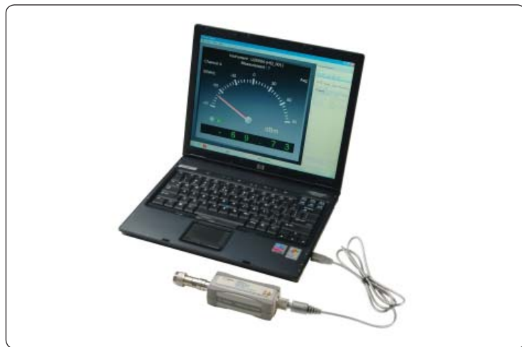
Figure 7 Instant interfacing of the U2000 Series with the Power Panel using a USB cable can be up to 5 meters long. Signal cable extension techniques for as long as 90 meters, using a LAN, will be covered later in this note.
