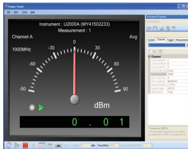
Figure 3 The N1918A Power Panel tool mimics an analog meter of a normal power meter instrument (only larger), and performs a wide variety of data computations.
