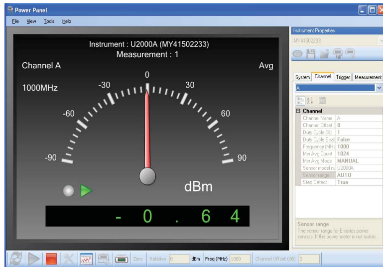
Figure 9 A typical soft front panel display for the basic N1918A Power Analysis Manager with an analog dial plus a digital readout.
